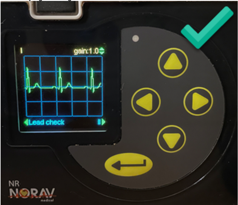
Figure 567. Verifying Recorder Data - Verifying ECG Signal
