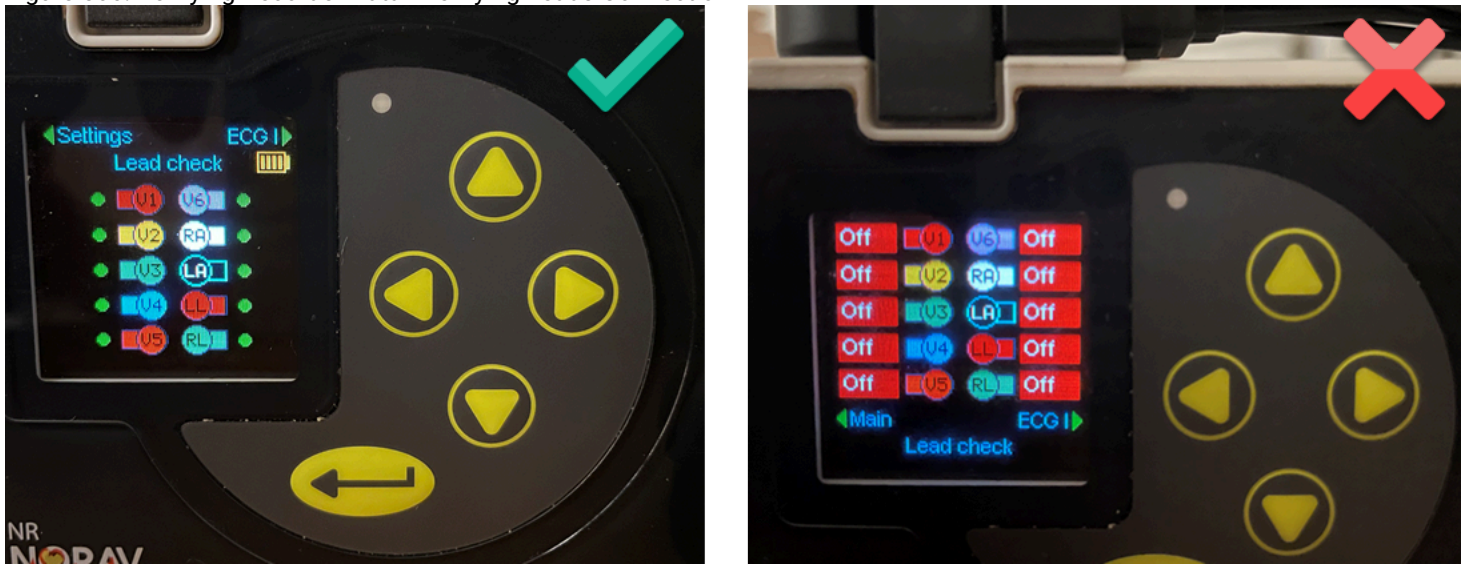
Figure 566. Verifying Recorder Data - Verifying Leads Connection
