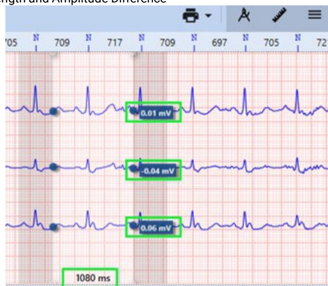
Figure 322. Strip View - Interval Length and Amplitude Difference
