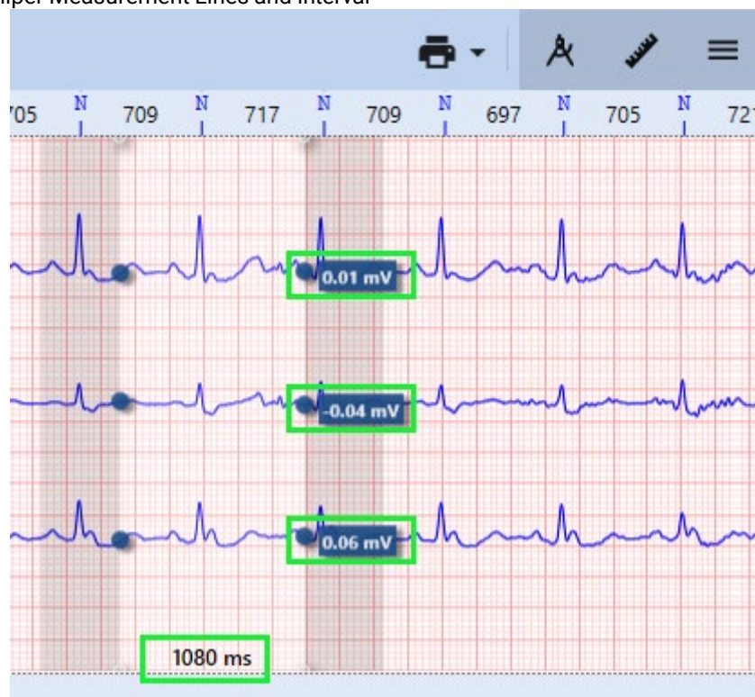
Figure 263. Strip View - Caliper Measurement Lines and Interval
